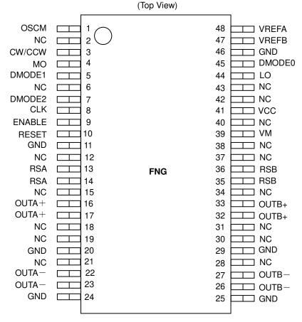
Please mount the exposed pad of the HTSSOP package to the GND area of the PCB.
