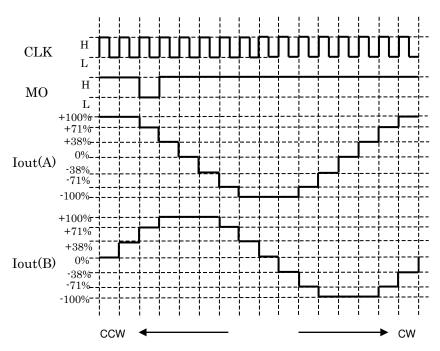
MO output shown in the timing chart is when the MO pin is pulled up. Timing charts may be simplified for explanatory purpose.
