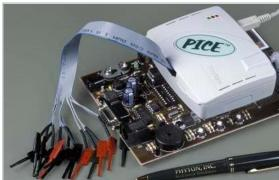
Intends to trace external signals from the target and to output syncronization impulses
