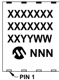
8-Lead MSOP (3x3 mm)
