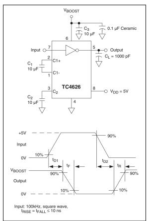
FIGURE 3-1: Inverting Driver Switching Time.
