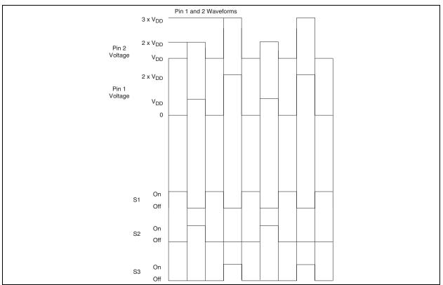
FIGURE 3-4: Position of Switches.
