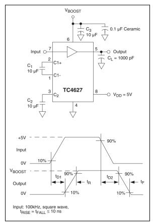
**FIGURE 3-2:** Noninverting Driver Switching Time.
