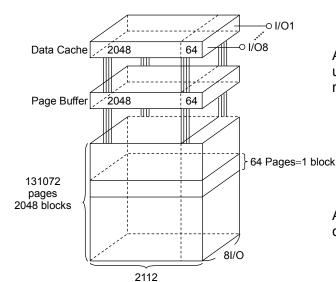
A page consists of 2112 bytes in which 2048 bytes are used for main memory storage and 64 bytes are for redundancy or for other uses.
