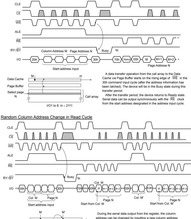
address can be changed by inputting a new column address using the 05h and E0h commands. The data is read out in serial starting at the new column address. Random Column Address Change operation can be done multiple times within the same page.
