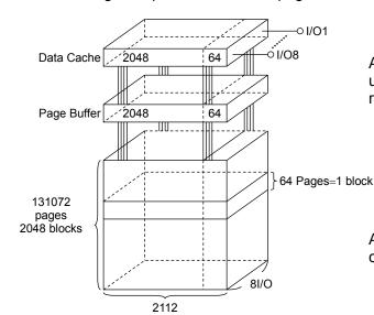
A page consists of 2112 bytes in which 2048 bytes are used for main memory storage and 64 bytes are for redundancy or for other uses.
