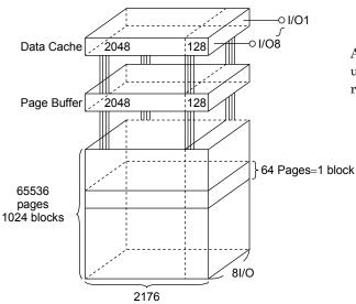
A page consists of 2176 bytes in which 2048 bytes are used for main memory storage and 128 bytes are for redundancy or for other uses.
