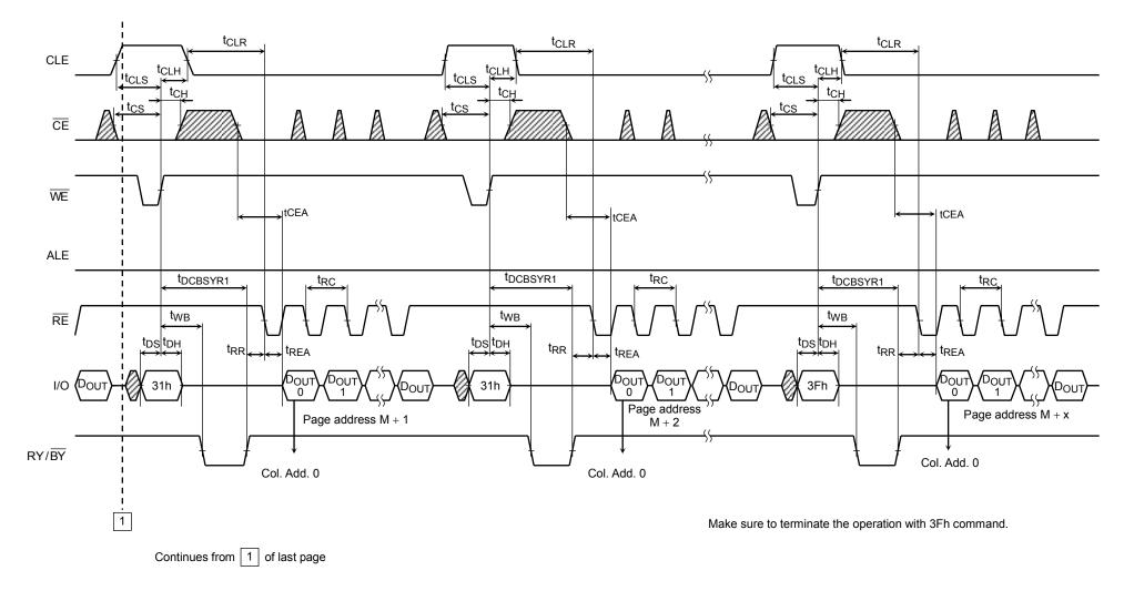
Column Address Change in Read Cycle Timing Diagram (1/2)
