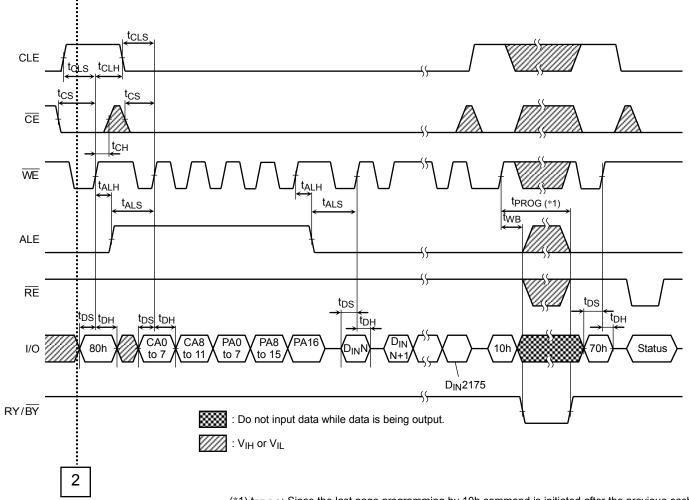
(\*1) t<sub>PROG</sub>: Since the last page programming by 10h command is initiated after the previous cache Continues from 2 of previous page program, the t<sub>PROG</sub> during cache programming is given by the following equation.
