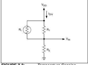
FIGURE 7-3: Temperature Sensing Circuit.
