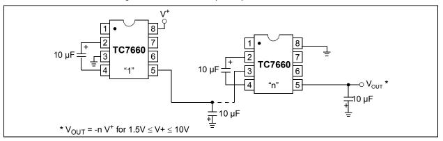
FIGURE 5-3: Increased Output Voltage By Cascading Devices.
