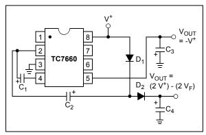
**FIGURE 5-7:** Combined Negative Converter and Positive Multiplier.
