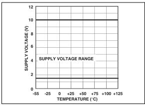
**FIGURE 2-1:** Operating Voltage vs. Temperature.
