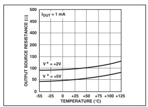
**FIGURE 2-5:** Output Source Resistance vs. Temperature.
