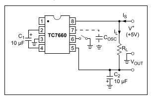
FIGURE 1-1: TC7660 Test Circuit.
