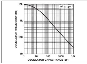
**FIGURE 2-3:** Frequency of Oscillation vs. Oscillator Capacitance.
