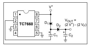
FIGURE 5-6: Positive Voltage Multiplier.
