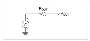
FIGURE 4-2: Switched Capacitor Inverter Equivalent Circuit Model.
