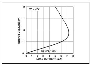
FIGURE 2-9: Output Voltage vs. Load Current.
