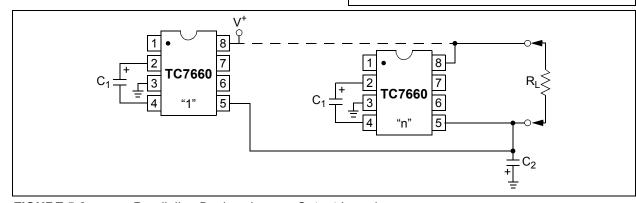
FIGURE 5-2: Paralleling Devices Lowers Output Impedance.
