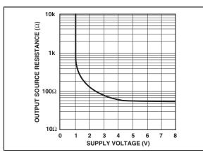
**FIGURE 2-2:** Output Source Resistance vs. Supply Voltage.
