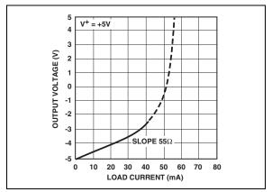
**FIGURE 2-10:** Output Voltage vs. Load Current.
