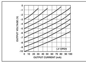
FIGURE 2-7: Output Voltage vs. Output Current.
