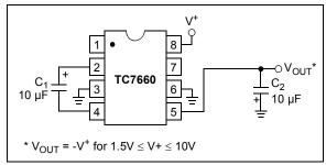
FIGURE 5-1: Simple Negative Converter.
