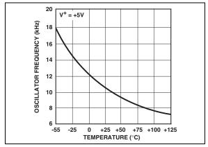
FIGURE 2-6: Unloaded Oscillator Frequency vs. Temperature.
