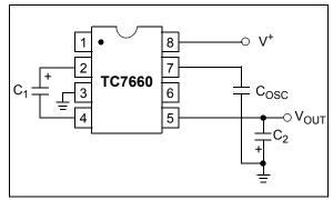
**FIGURE 5-5:** Lowering Oscillator Frequency.
