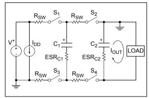
FIGURE 4-3: Non-Ideal Switched Capacitor Inverter.
