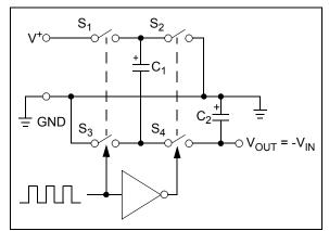
FIGURE 4-1: Ideal Switched Capacitor Inverter.
