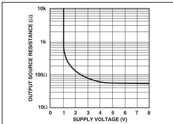
**FIGURE 2-2:** Output Source Resistance vs. Supply Voltage.
