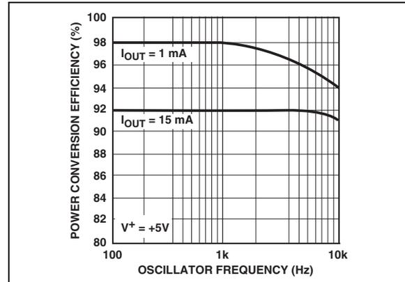
**FIGURE 2-4:** Power Conversion Efficiency vs. Oscillator Frequency.
