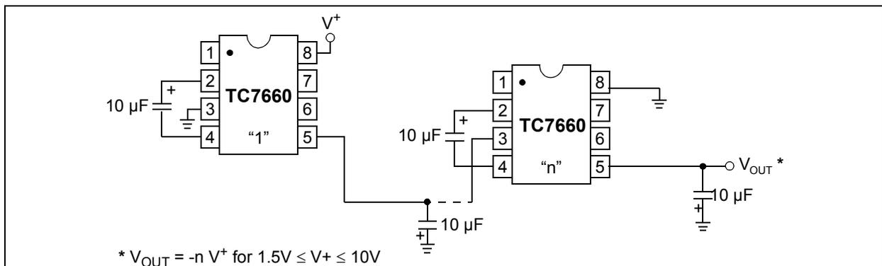
**FIGURE 5-3:** Increased Output Voltage By Cascading Devices.
