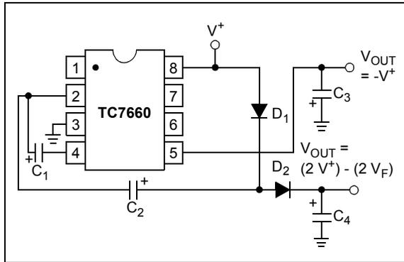
**FIGURE 5-7:** Combined Negative Converter and Positive Multiplier.
