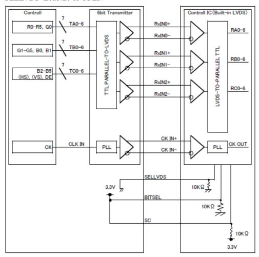
$\mbox{\ensuremath{\mbox{\$SELLVDS}}}$  signal line has 10 k  $\Omega$  -pulldown resister.
