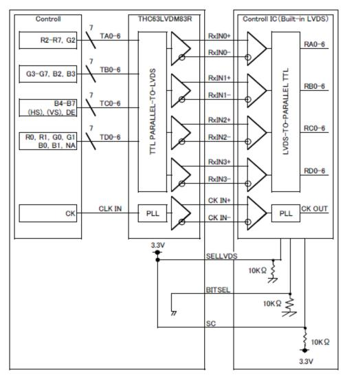
$\mbox{\ensuremath{\mbox{\$}}{SELLVDS}}$  signal line has 10 k  $\Omega$   $\,$  pulldown resister.
