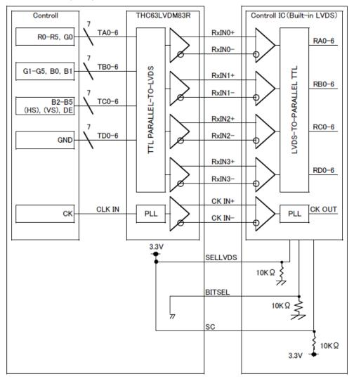
$\mbox{\ensuremath{\,\raisebox{-.3ex}{$\times$}}} SELLVDS$  signal line has 10 k  $\Omega$   $\,$  pulldown resister.
