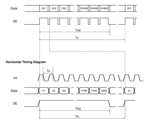
8-2. Input Data Signals and Display position on the screen
