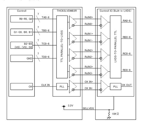
When using "6-bit Transmitter", please connect the unused channel of the control IC receiver as described in the diagram below.
