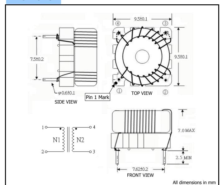
**SPECIFICATIONS** Pin 1-2:  $33.3\mu H \pm 20\%$ Pin 3-4:  $33.3\mu H \pm 20\%$ Inductance Test Condition: 100KHZ/50V Measurement Instrument: HP 4263B LCR Meter DCR(Max):  $8.5m\Omega$ **Impedance** Measurement Instrument: HIOKI 3540 mΩ Hitester IDC(Max): 4A Rated current Measurement Instrument: Agilent 34401A Meter Rated voltage 500Vdc -40°C ~ +105°C Operating temperature Recommended Through Hole Φ 0.8 mm
