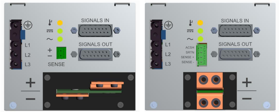
Figure 1b. Rear View of TCP3500-1024G (left) and TCP4000-H090 (right) - Connectors Position
