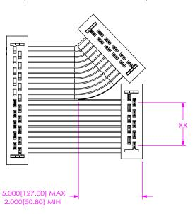
"XX" = NO. OF CONDUCTORS BROKEN OUT FROM THE FIRST POSITION. AN EVEN NUMBER POSITION BREAKOUT MUST BE SELECTED FOR A DOUBLE ENDED ASSEMBLY AND THE BREAKOUT ENDS MUST BE EQUAL TO THE FULL POSITION CONNECTOR.
