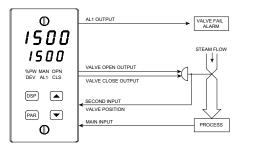
The motorized valve positioner controls the position of a valve directly, by use of "open" and "close" control outputs. The slidewire feedback signals of the valve may optionally be connected to the controller. Alternatively, the controller may be configured for linear input valve control using the 4 to 20 mA DC output.
