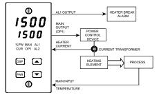
The Heater Current Monitor serves as a heater element fail sentry, so operators can take corrective action before significant process errors occur in the event of a failure. The actual heater current can be viewed in the secondary display and/or a heater break alarm output can be programmed.
