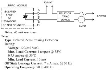
Protection: Internal Transient Snubber, Fused
