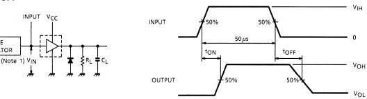
Note 1: Pulse width 50 µs, duty cycle 10% Output impedance 50  $\Omega$ ,  $t_f \leq 5$  ns,  $t_f \leq 10$  ns Note 2: CL includes probe and jig capacitance
