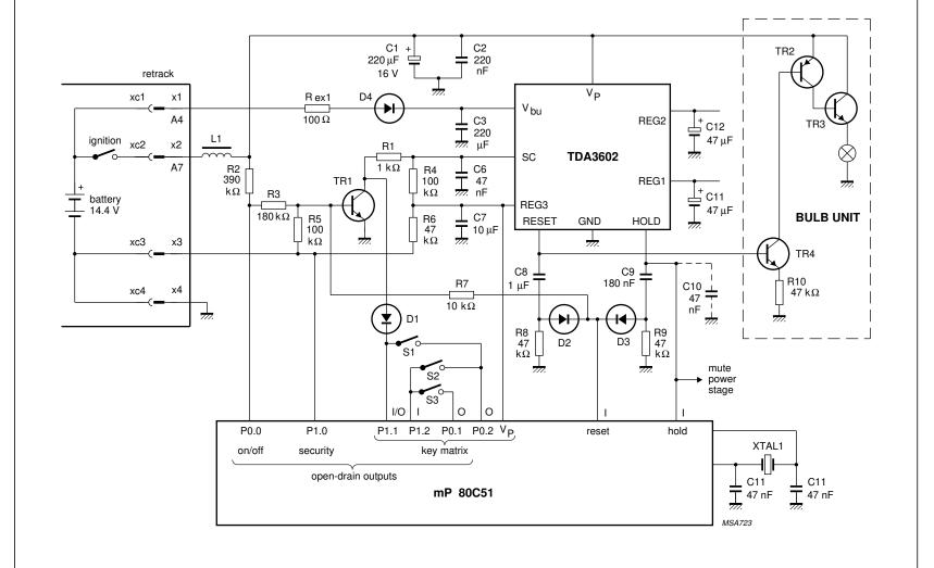
Fig.11 Application with all features of semi on/off logic.
