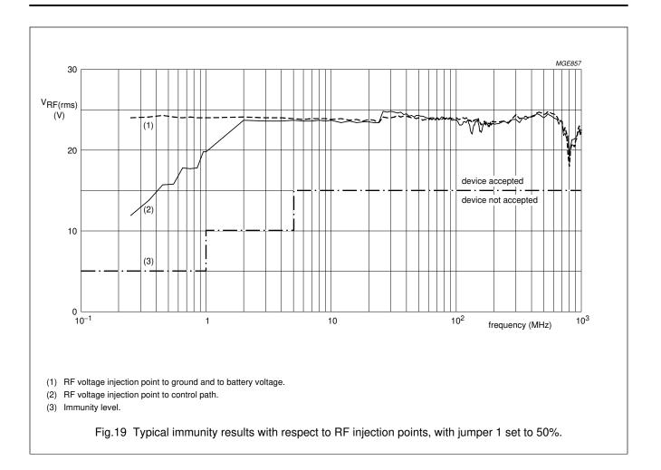
The typical immunity results of the TDA3629T are shown in Fig.18. The RF voltage was injected into the control line (see also Figs 13 and 14). This injection point is the most sensitive one that could be found. This is underlined by the comparison results shown in Fig.19.
