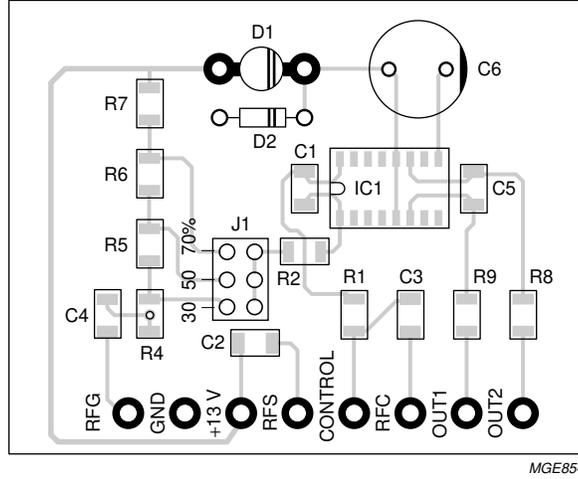
Fig.15 Component placement of the printed-circuit board.
