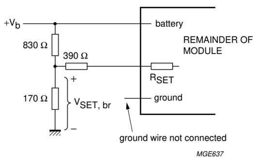
The 170  $\Omega$ , 830  $\Omega$  and 390  $\Omega$  resistors form the setting potentiometer in its worst case position. The given situation (combination of  $V_b$ ,  $R_{SET}$  and the position of the set potentiometer) forms the worst case situation. The given maximum of  $\Delta V_{SET}$  guarantees that any other module, connected to the same set potentiometer, will not start to activate its motor, when its motor switch-on level is higher than  $0.01V_b$  ( $R_{SET} \geq 20$  k $\Omega$ ).
