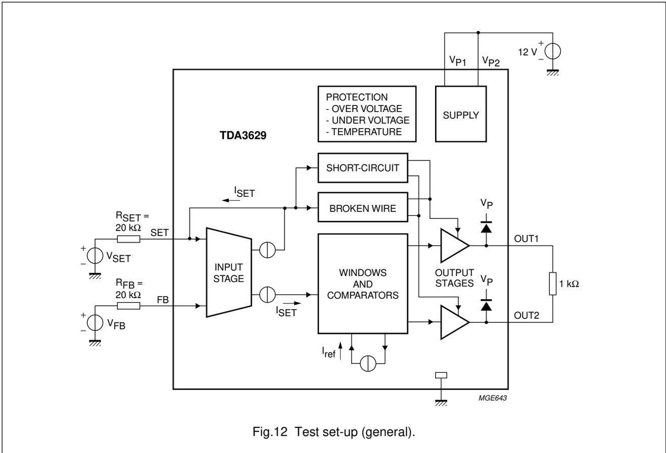
Fig.12 Test set-up (general).
