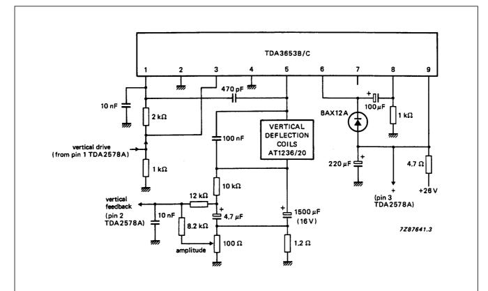
Note to deflection coils AT1236/20: L = 29 mH, R = 13.6 Ω; deflection current without overscan is 0.82 A peak-to-peak and EHT voltage is 25 kV.
