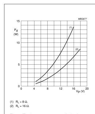
Fig.7 Total worst case power dissipation as a function of supply voltage.
