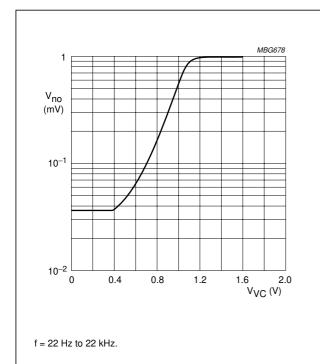
Fig.9 Noise voltage as a function of volume control voltage.
