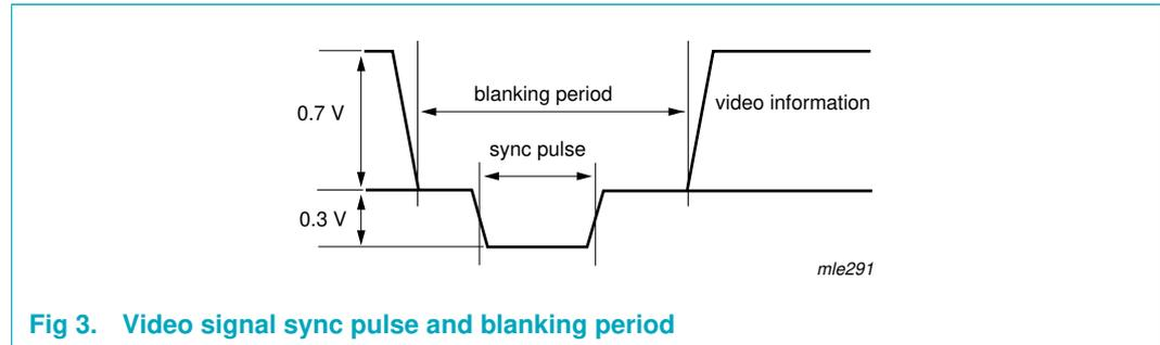
Fig 3. Video signal sync pulse and blanking period
