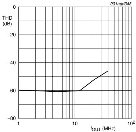
Fig 7. THD as a function of  $f_{OUT}$ , typical values
