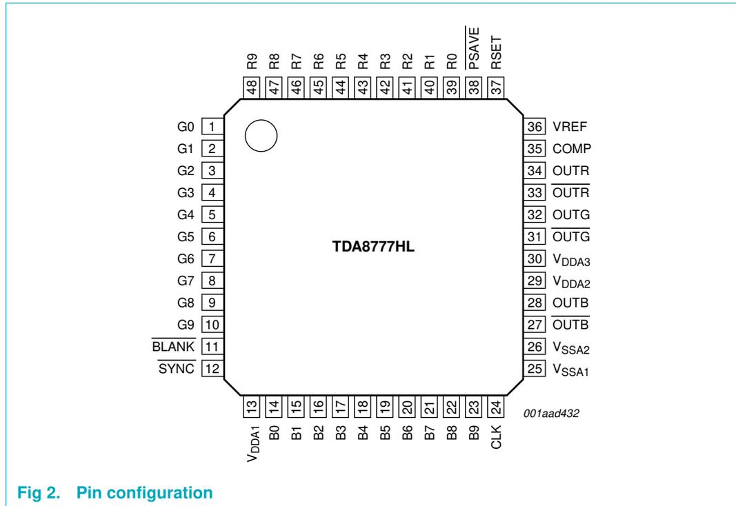
Fig 2. Pin configuration
