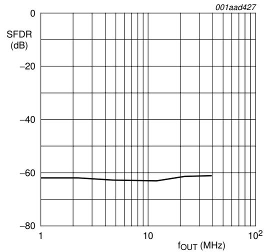
Fig 8. SFDR as a function of  $f_{OUT}$ , typical values
