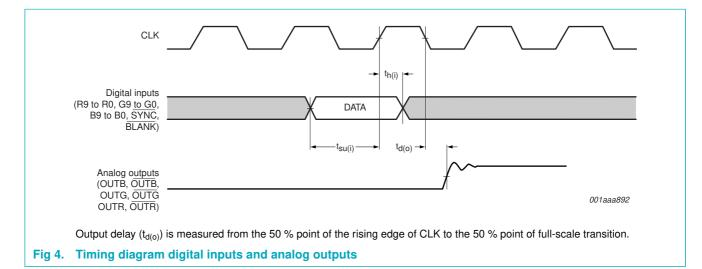
Triple 10-bit video DAC, up to 330 MHz sample frequency
