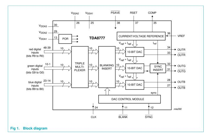
Triple 10-bit video DAC, up to 330 MHz sample frequency
