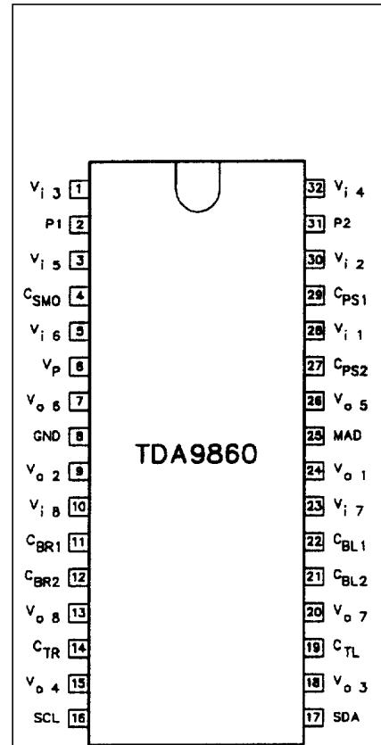
Fig.2 Pin configuration.
