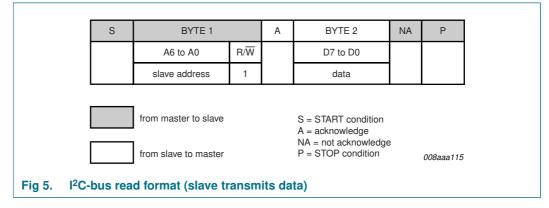
The master generates an acknowledge when it has received the data word READ. The master next generates an acknowledge, then slave begins transmitting the data word READ, and so on until the master generates an acknowledge-not bit and transmits a STOP condition.
