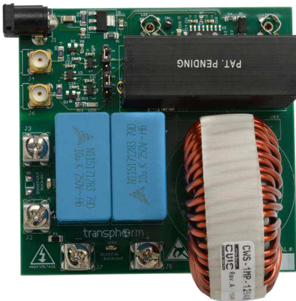
Figure 1. Half-bridge evaluation board
