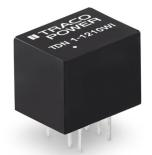
The TDN 1WI Series comprises 1 Watt fully regulated, high performance DC/ DC converters. They come in a compact cubical package of only 1.23 cm<sup>3</sup>. Full load operation is reliable up tp 90°C environment temperature. With 1'600 VDC I/O-isolation voltage, external On/Off, and short current protection they cover a wide range of application when space is limited. The input of the converters is designed for a wide voltage range (4:1) and minimum load is not required. The
