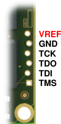
Figure 24: JTAG connector J2.
