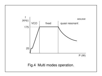
The next converter stroke is started only after demagnetization of the transformer current (zero current switching), while the drain voltage has reached the lowest voltage to prevent switching losses (green function). The primary resonant circuit of the primary inductance and drain capacitor ensures this quasi-resonant operation. The design can be optimized in such a way that zero voltage switching can be reached over almost the universal mains range.
