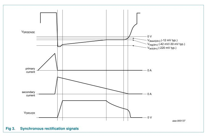
The level of the driver regulation voltage  $V_{reg(drv)}$  can be selected using the SELREG pin. When this SELREG pin is grounded, the typical  $V_{reg(drv)}$  equals –42 mV. When the SELREG pin is left open, the  $V_{reg(drv)}$  level equals –30 mV.
