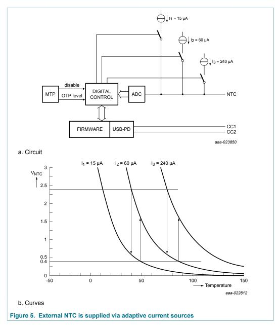
The voltage at the NTC pin is measured via an internal A-to-D converter. If the voltage on the NTC pin drops to below 400 mV, the source current of the pin is increased. If the voltage on this pin exceeds 2.4 V, the source current of the pin is decreased. In this way, the temperatures are measured with a better than 5  $^{\circ}$ C accuracy for a range of 0  $^{\circ}$ C to > 120  $^{\circ}$ C when using a typical external resistor.
