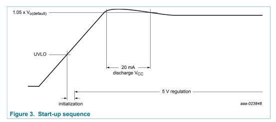
The TEA19032BT operates on supply voltages up to 21 V. The voltage on the VCC pin is used to detect an OVP and UVP. The OVP and UVP level are set as a percentage of the requested output voltage level.
