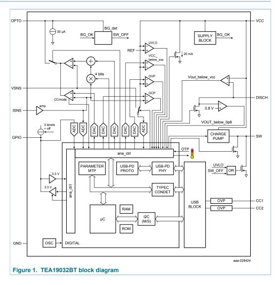
USB-PD 2.0/USB-PD 3.0/QC 4 controller for SMPS
