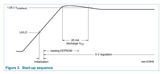
The TEA19051BTK operates on supply voltages up to 21 V. The voltage on the VCC pin is used to detect an OVP and UVP. The OVP and UVP level are set as a percentage of the requested output voltage level.
