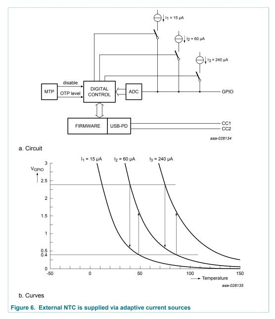
The voltage at a GPIO pin is measured via an internal A-to-D converter. If the voltage on the GPIO pin drops to below 400 mV, the source current is increased. If the voltage on the GPIO pin exceeds 2.4 V, the source current is decreased. When a 47 k $\Omega$  NTC resistor with a Beta of 4108 is used, the temperature is accurately measured with a better than < 5 °C accuracy within a range of 0 °C to > 120 °C.
