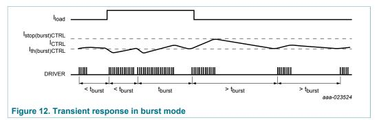
Even though the burst-mode regulates toward a target repetition frequency, the actual repetition rate is lower than the target because of the discrete number of switching cycles. Increasing or decreasing the number of pulses results in a step change in the burst repetition frequency.
