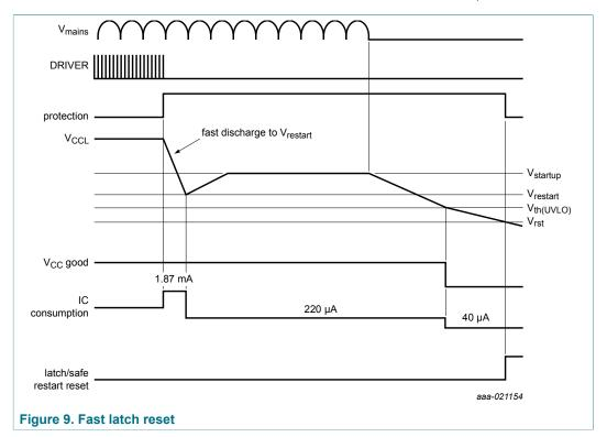
Using a 10  $\mu$ F total capacitance value on the VCCL and VCCH pins, the fast latch reset time is below 0.6 s. If the mains is not shorted but removed, a discharge of the X-cap can cause an additional delay time.
