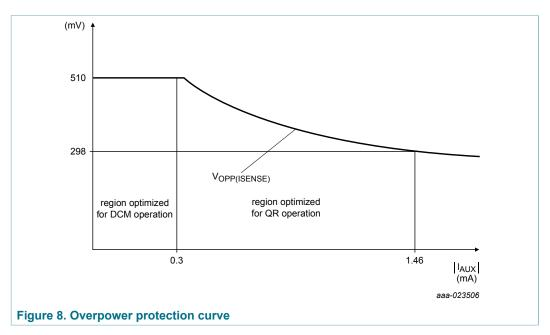
During system start-up, the maximum timeout period is lowered to 40 ms. When the output voltage is within its regulation level, the maximum timeout period returns to 200 ms, limiting the output power to a minimum at a shorted output. Shortening the overpower timer ensures that the input power of the system is limited to < 5 W at a shorted output.
