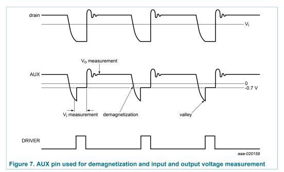
When the external MOSFET is switched on, the voltage at the auxiliary windings reflects the input voltage. The AUX pin is clamped to -0.7 V. The output current is a measure of the input voltage. This current value is internally used to set the overpower limit on  $V_{\text{sense(ipk)}}$ . The demagnetization, valley and output voltages are measured as a voltage on the AUX pin. In this way, the input voltage measurement and OVP can be adjusted independently.
