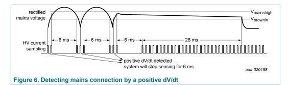
If a positive dV/dt is not detected for 28 ms, the system assumes that the mains is disconnected. In that case, the HV pin is continuously pulled to ground, discharging the external X-capacitor.
