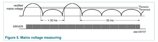
When the mains voltage is measured by pulling the HV pin to ground, the digital control calculates if there is a positive dV/dt at the mains. A positive dV/dt implies that a mains is connected.
