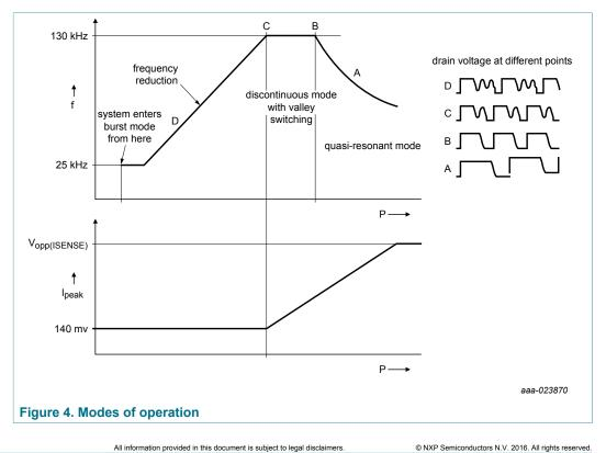
At high output power, the converter operates in QR-mode. Each converter cycle starts after the demagnetization of the transformer and the detection of the valley at the end of the previous cycle. In QR-mode, switching losses are minimized because the external MOSFET is switched on while the drain-source voltage is minimal.
