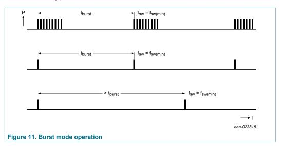
To achieve a good transient response at an increased output load, the system starts switching immediately when  $I_{CTRL}$  drops to below  $I_{start(burst)}$ . It keeps switching until the optocurrent exceeds the level of  $I_{start(burst)CTRL}$  (100 µA). On the other hand, to achieve a good transient response at a decreased output load, the system stops switching immediately when the optocurrent exceeds the level of  $I_{stop(burst)CTRL}$  (200 µA) at a
