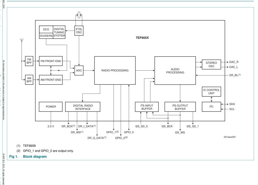
**DSP-based radio tuner one-chip**
