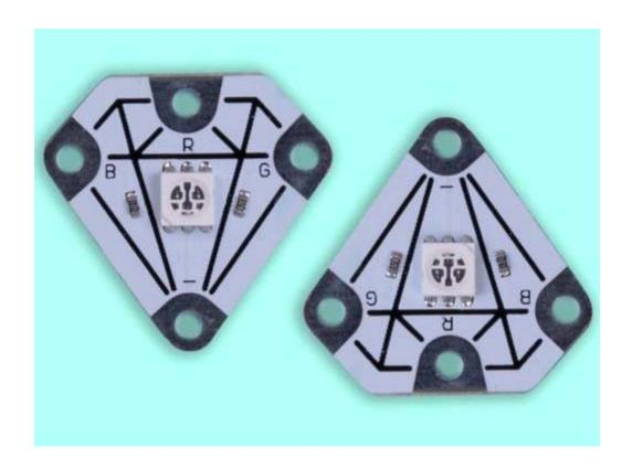
Two diamond-shaped, sewable LED boards that are colour-changeable! They can be connected to light up in red, blue, green, or any combination of those colours!
