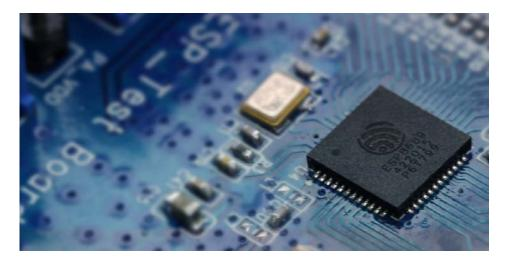
Compared to the arduino ESP8266 (the previous generation), the ESP32 has a significant performance improvement. It is equipped with a high-performance dual-core Tensilica LX6 MCU. One core handles high speed connection and the other for standalone application development. The dual-core MCU has a 240 MHz frequency and a computing power of 600 DMIPS.
