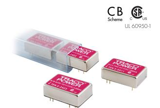
The TEN 5 Series is a range of DC/DC-converter modules with wide input range of 2:1. State of the art SMD-technology guarantees a product with very high reliability and good cost /performance ratio. I/O-isolation of 1'500 VDC together with conducted noise compliance to EN 55022-A and FCC level A makes these converters ideal for a wide range of applications in communications, mobile battery powered equipments and industrial systems.
