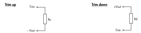
Nominal output voltage at open Trim input Ru, Rd for adjustment
