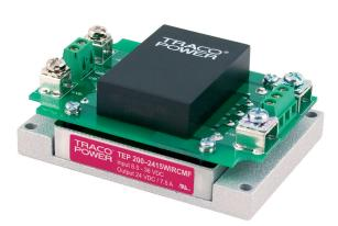
The TEP 200WIR Series is a family of isolated high performance dc-dc converter modules with ultra-wide 4:1 input voltage ranges. They come in chassis mount version with screw terminal block and with integrated EMI input filter to meet EN 55032 class A. A very high efficiency allows full power operation at 25°C with only 100 LFM air flow couling and operation at 60°C with only 40% power derating.
