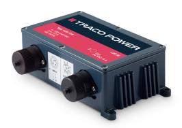
These power supplies have been designed particularly for applications in extreme environments. The rugged die-cast aluminium housing is water, ice, oil and dust resistant in compliance with IP67 and NEMA 4X standards. The metal case works as an efficient heatsink allowing full power operation at up to +60°C ambient temperature (no fan required). With a shock and vibration proof construction the power supplies can be mounted directly on a machine.
