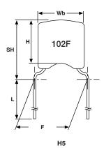
Component outline for lead spacing 5.0 mm  $\pm$  0.8 mm (flat bent leads)
