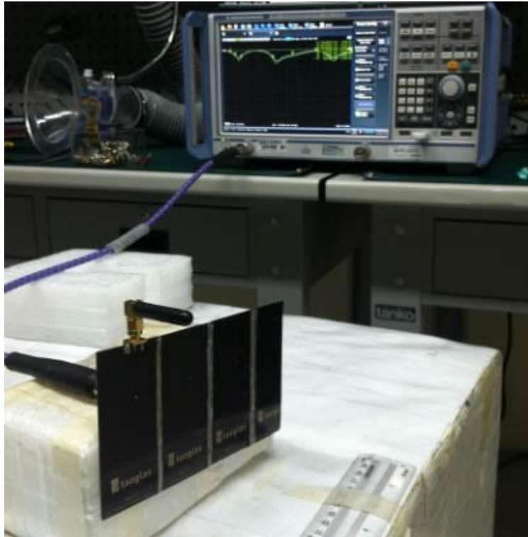
Figure 1. Impedance and VSWR measurements
