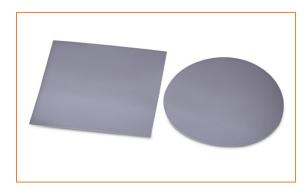
TG-C105BK is a pressure sensitive adhesive (PSA) tape that has good electrical conduction in the X-Y-Z-axis direction. It has low contract resistance and superior adhesive force, which can shield electromagnetic interference (EMI) effectively. TG-C105BK can be supplied as die cut parts or in roll form.
