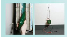
Non-Contact probe audibly identifies selected wire or cable. Easily trace wires from source to termination.
