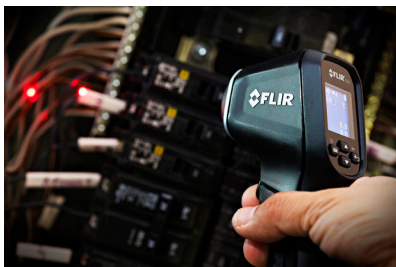
Easily identify measurement location with built-in laser
